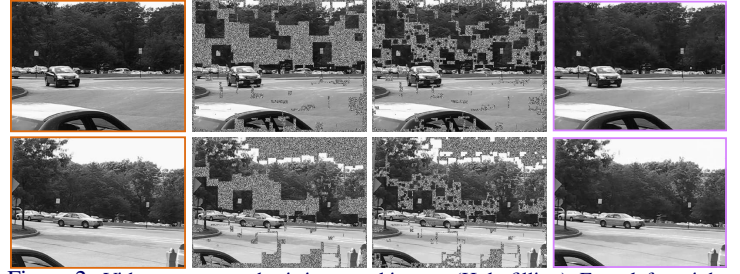
Figure 2: Video texture synthesis in natural images (Hole-filling). From left to right: (i) Last frame (5th) of input video, (ii) Structure regions, (iii) Structure / Texture regions, (iv) Synthesized frame (our result).
