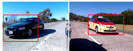
Figure 8: Sample detection results of the vehicles in the right and left blind spots.
