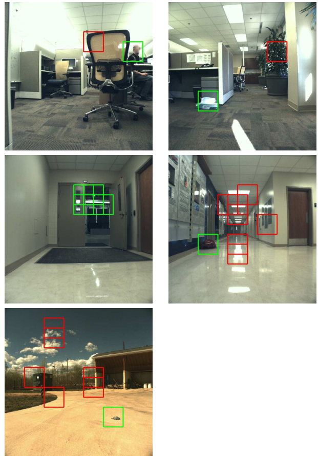
Figure 7. Anomalies detected in the environments. In the figure, green rectangles show correctly detected anomalies; red rectangles show false positives. Any detected faces are blurred to preserve privacy.
