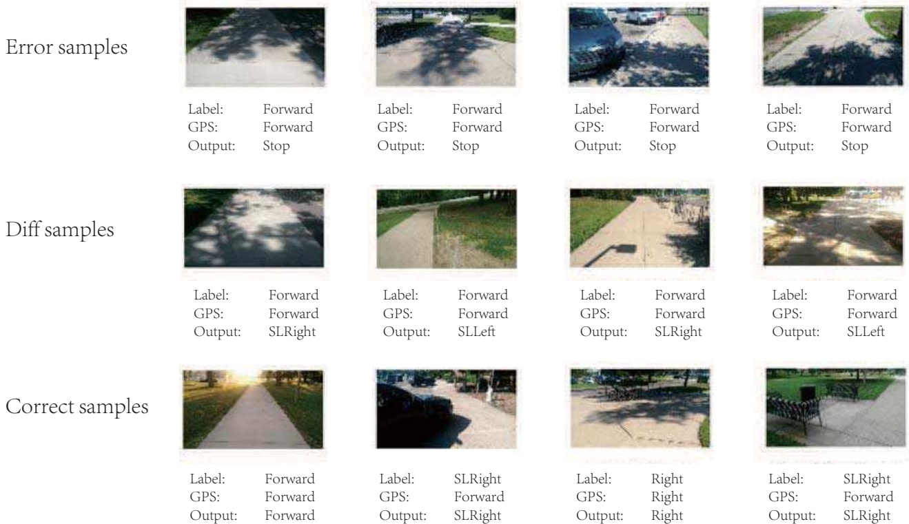
Figure 8. Testing samples from regular testing session. Sharp contrast caused by over-casting shadows was the biggest challenge to the performance of the network. The observed errors are all caused by shadows with sharp contrast and irregular shapes. Sec.4.2 discusses how this issue can be resolved. Diff is short for different from supervisor's intention .
