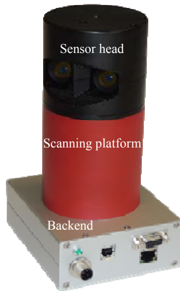
Figure 1: The realized 360° HDR depth camera
