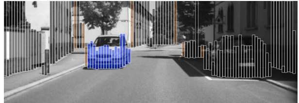
(d) Segmentation of the Stixel World into static background/infrastructure and moving objects. The color represents a group of connected Stixels with similar motion. Brown Stixels are flagged as potentially inaccurate.
