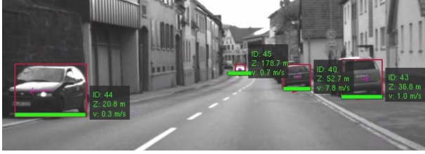
Figure 8: Full-range (0 m - 200 m) vehicle detection and tracking example in an urban scenario. Green bars indicate the detector confidence-level.
